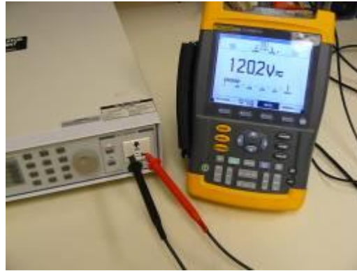
Figure 6b: Voltage measurement of 120.2VAC between line and neutral output
