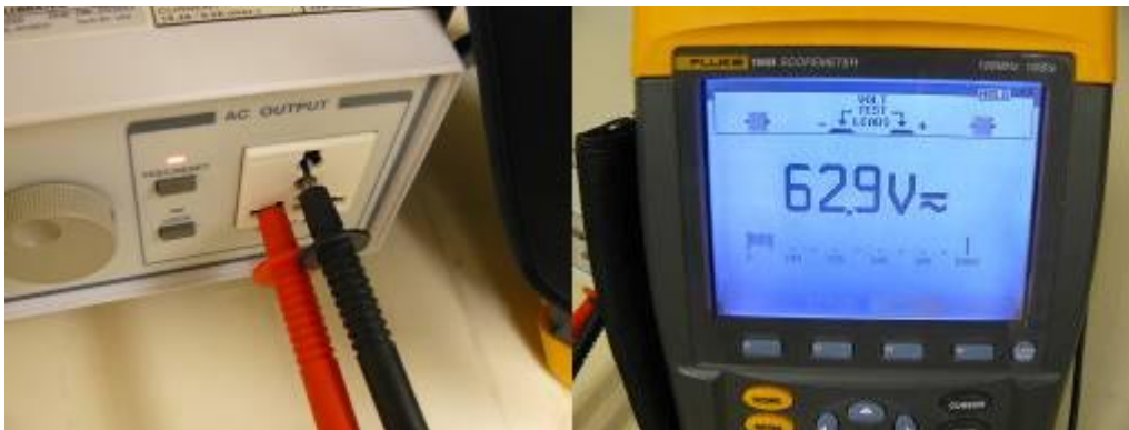
Figure 6d: Voltage measurement between line and ground
